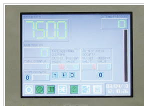
TOUCH SCREEN Clear readings ensure quick fault finding and machine operation. Cutting pressure gauge checks cutting pressure and over-cutting pressure.
