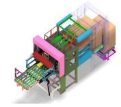
Pile goes up automatically via the Elevator.
