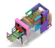
Sheets can be inverted or passed through to be stacked.
