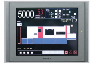
TOUCH SCREEN Clear and simple readings ensure quick diagnosis. Operator-friendly controls for easy adjustments. Machine position and running speed displayed.
